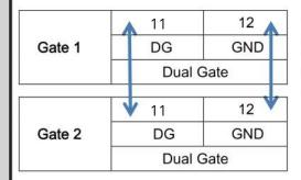
Connecting the terminal (DG and GND) on both control boards with 2 x 0.75m cable (see left figure), which could open both gates. Transmitter only needs to do the system learning with one motor. When pressing the transmitter, both motors will operate at the same time.
